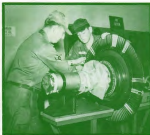
Replacing turbine wheel buckets.
